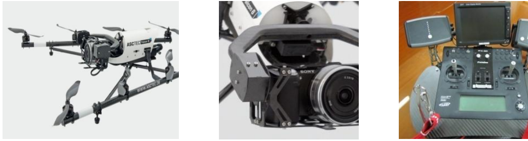
Fig. 1 UAV (Falcon 8) and facilities used for aerial photography
