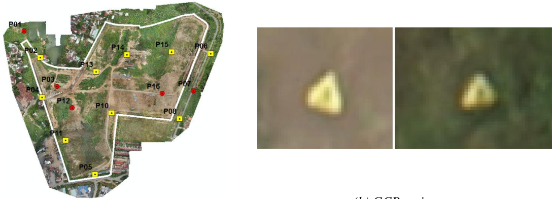
Fig. 3. (a) GCP distribution on the depot
